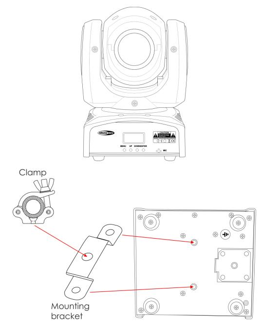
The Kanjo can be placed on a flat stage floor or mounted to any kind of truss with a clamp.
