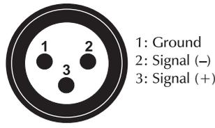
If you are using the recommended FUTURELIGHT-controllers, you can connect the DMX-output of the controller directly with the DMX-input of the first fixture in the DMX-chain. If you wish to connect DMX-controllers with other DMX-outputs, you need to use adapter-cables.
