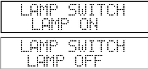
The controller is able to simply switch the glow-lamp of the controlled units on and off – only if the unit has such a function and a special lamp function was set at the installation! By keeping the LEFT/RIGHT buttons pressed simultaneously the controller switches to lamp mode. At that time switching-on and switching-out values can be forwarded to the units with buttons 1-16. If you press
