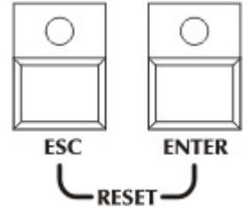
The controller is able to reset the controlled units if the unit has such a function and a special reset function was set during the installation! In case you keep the ESC-ENTER buttons pressed simultaneously the controller switches to reset mode. Then the reset command can be forwarded to the units with buttons 1-16. The controller sends the reset command to the units until the button is kept pressed! You can log off from the setup pressing the ESC or ENTER button.
