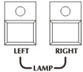
the UP button, the LED starts flashing, signaling that the glow-lamps can now be turned on with buttons 1-16. The controller sends switching-on values to the units while you keep that button pressed! If you press the DOWN button, its LED starts flashing, signaling that glow-lamp switching-out commands can be sent to the units with buttons 1-16. You can log off from the setup by pressing the LEFT or RIGHT button.
