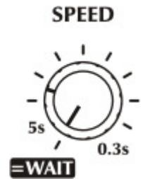
to the new position within the time of the scene time. At the moment of their stop the next scene begins to load. So during the program running the beams will never wait at the same time. In the right upper line the display indicates the SPEED value is the same as the WAIT value at present.
