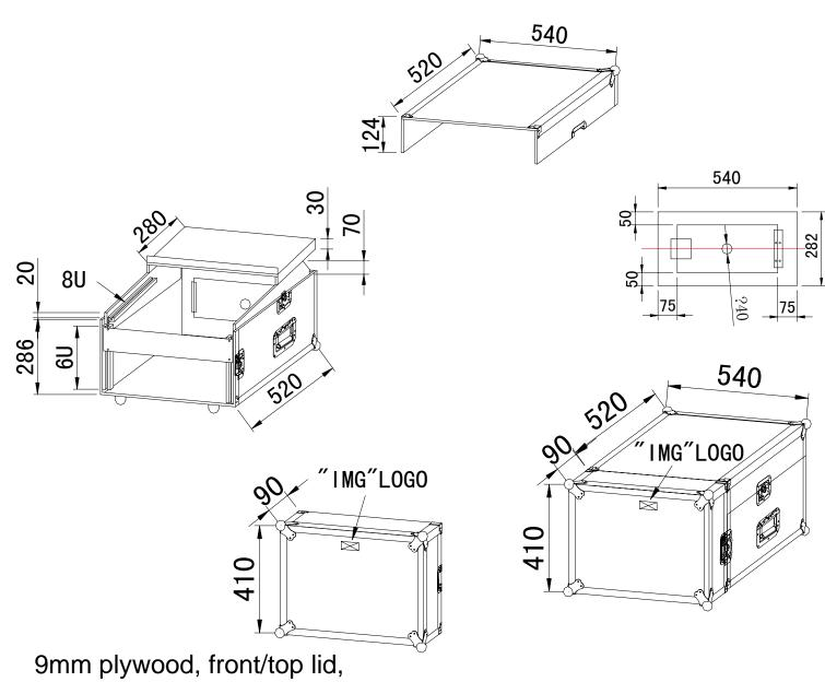
9mm plywood, front/top lid, aluminum rack rail, 1pcs 2U rack panel, 5 latches, 2 handles, 4 rubber feet.
