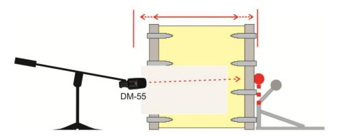
• Place the DM-55 in front of the hole in the drumhead. Aim the microphone at the place where the beater hits the rear drumhead. If you feel that your sound lacks brilliance, move the DM-55 closer to the beater.
