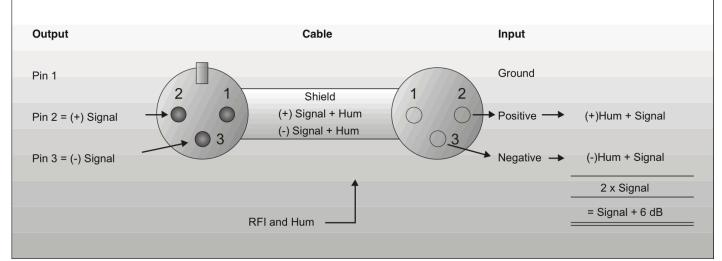
Compensation of interference with balanced connections
