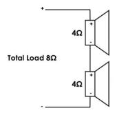
In a low impedance system, the total speakerload should always match the amplifier impedance. This to avoid overloading the amplifier.
