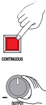
In the continuous mode, the fog machine will emit fog continuously. The output volume is adjustable.
