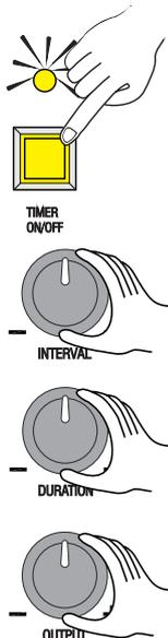
In the timer mode, the fog machine will automatically emit fog. The time intervals, duration and fog volume are adjustable.
