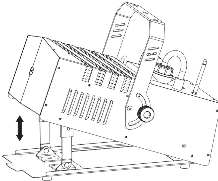
The output angle can be adjusted by raising the device via the two supporting legs. The legs can be raised up to five steps.
