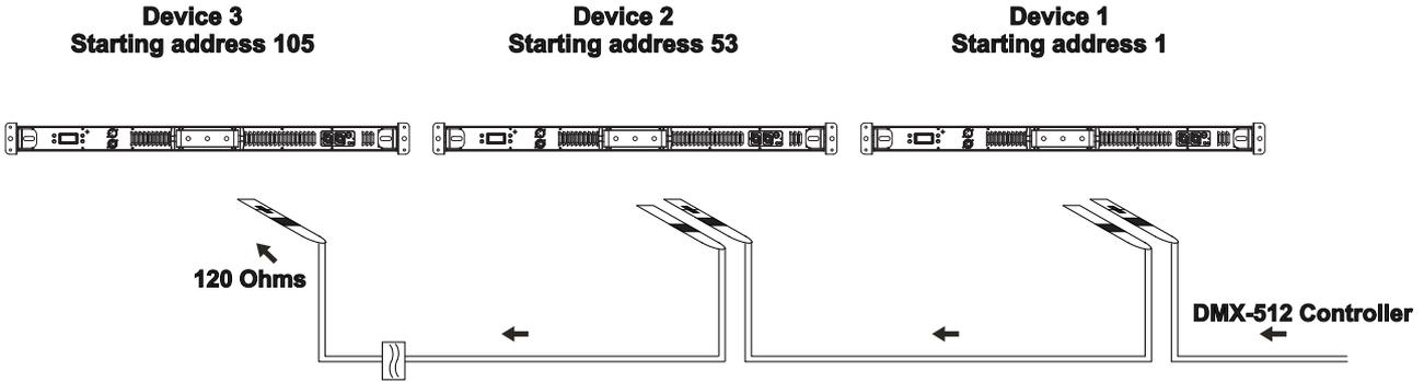
**! The wires must not come into contact with each other, otherwise the fixtures will not work at all, or will not work properly. !**
