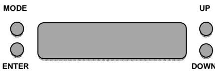
Browse through the menu by pressing Mode. Press Enter in order to select the desired menu. You can change the selection by pressing Up or Down. Press Enter in order to confirm. You can leave every mode by pressing Mode. The functions provided are listed in the following sections.
