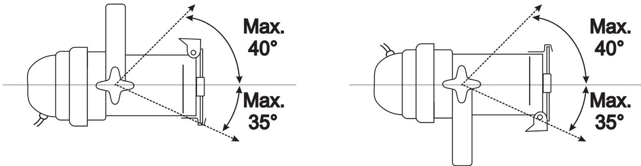
Adjust the desired inclination-angle via the mounting-bracket and tighten the fixation screws.
