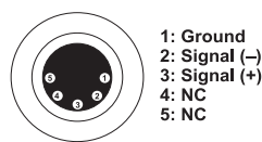
DMX-output XLR mounting-socket:
