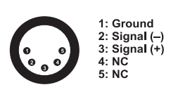
DMX-input XLR mounting-plug:
