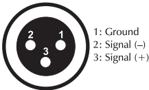
DMX-output XLR mounting-socket:
