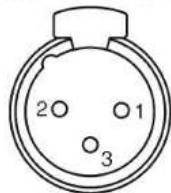
DMX - output XLR mounting-sockets (rear view):
