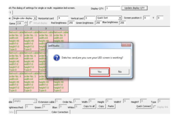
Your led screen is now patched. Be ware that the led screen will only show a part of your input because the pixel resolution of the input is much bigger then the total of pixels (=leds) on your led screen.
