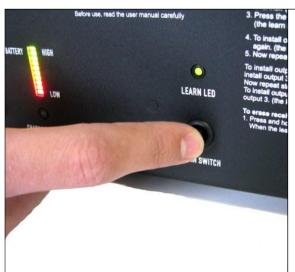
To make the Shot Base Wireless react to a remote 4/8 turn on the remote and press the LEARN SWITCH on the Shot Base Wireless, now the LEARN LED will blink once. This means output 1 can be programmed to button on the remote.
