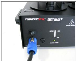
When the Shot Base Wireless is fully charged (the LED CHARGING BATTERY is green) u can choose to unplug the Shot Base Wireless and use it wireless
