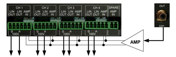
The spare amplifier can carry out a special task in such a system. In case the system is only set up as described with one amplifier and e.g. during regular operation, the background music is only played in circuit 1, the speakers of the circuits 2-4 will not be monitored. The spare amplifier can then carry out this task. For this, the function **RELAY** is available in the routing menu.
