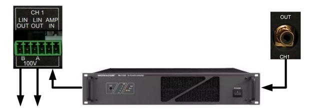
The input of the second amplifier is connected to the spare output (spare OUT) of the MEVAC-4. The 100 V output of the spare power amplifier is connected to the corresponding general feeding point at the rear side of the MEVAC-4.
