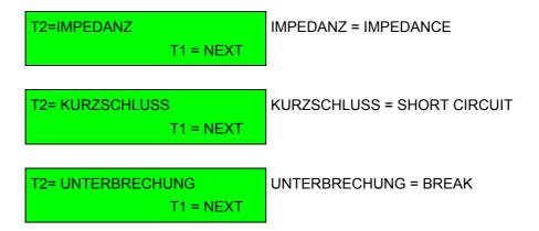
To insert volume controls into one circuit, the impedance deviation test of the corresponding circuit must be switched off. Also connect the emergency priority relays of the volume controls. A 1  $k\Omega$  terminating resistor has to be connected to the speaker line, if volume controls are used which switch themselves off at the position off/zero. Otherwise, the error message BREAK will appear.
