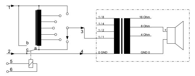
When the control is set to its maximum position at the installation run and is then turned to 50 % during operation, it will be identified as a deviation of more than 20 % and a corresponding error message will be displayed. In case the attenuator is in operation during the installation run, the connected speaker circuit may be identified as uninstalled.
