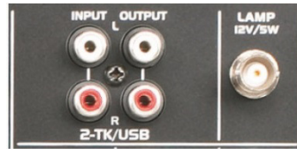
Fig. 4.15 RCA connectors and lamp socket
