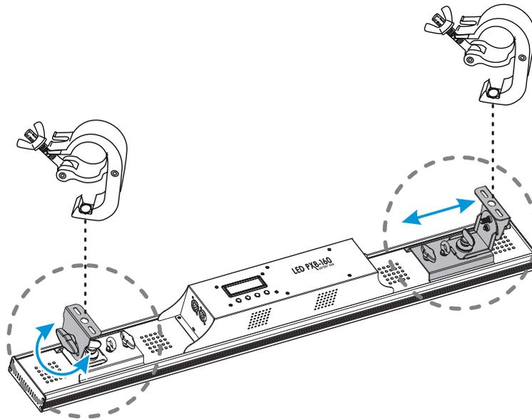
The LED bar comes with two adjustable mounting brackets which serve as a floor or wall mount support. The brackets can be slid to the left and right and adjusted to different angles. You may also attach clamps via M10 screws directly to the brackets for truss installation.
