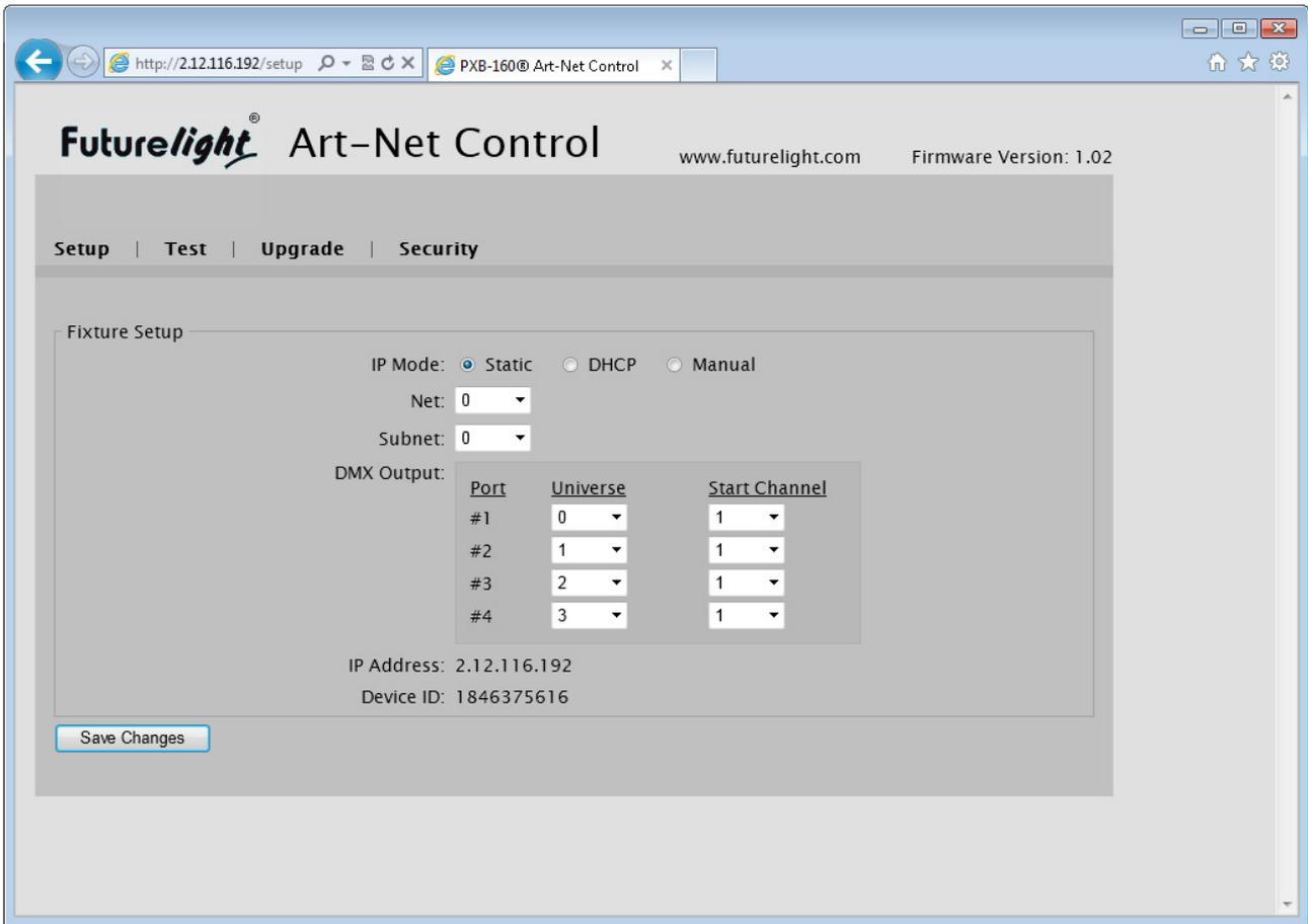
The LED PXB-160 Artnet Bar features a web interface to control the fixture with a standard browser remotely, instead of any third-party software. You can use the web interface to configure the fixture, test the output, and upgrade the firmware.
