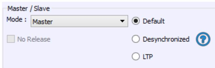
The Stand Alone mode allows to choose 1 interface and to define this interface as Master from the interface list, it is possible to choose only one to be the Master, all the other one will be configured as slave by default. The interfaces are always ordered by serial number ascending order.
