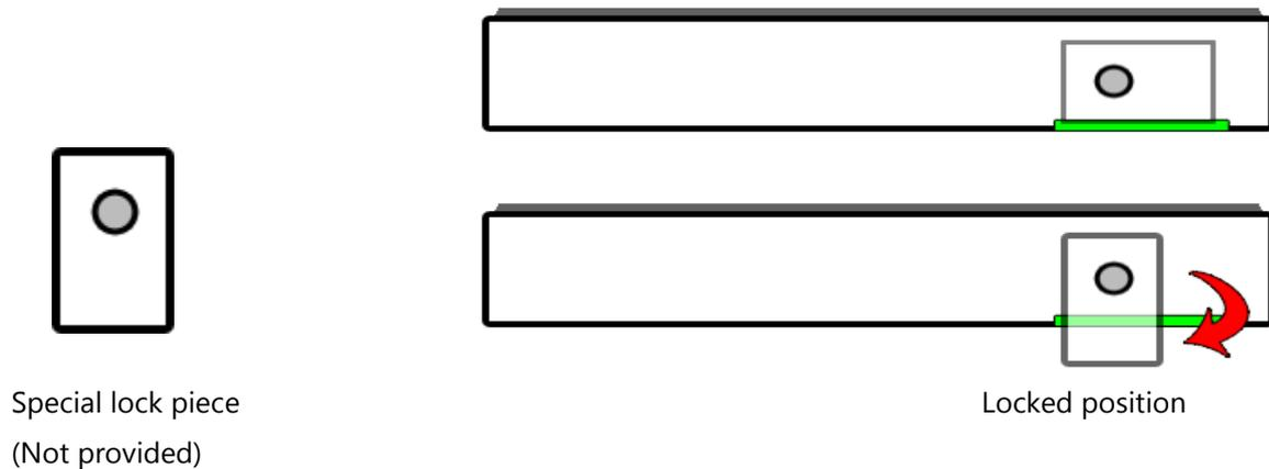
Thanks to that lock, it's now **not possible** to slide back the switch box screws to the plain holes of the SLIM case.
