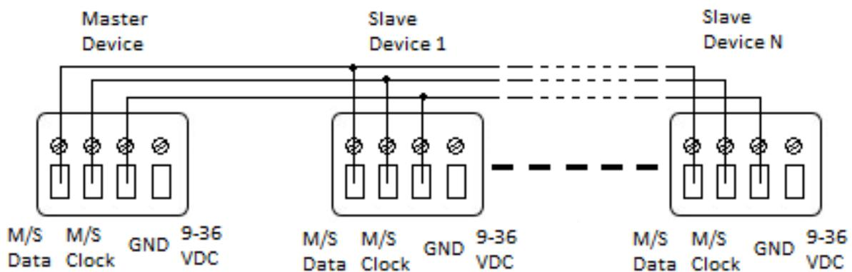
Interfaces configured as slave will strictly follow the clock, triggers and information providing by the master interface. Only one master interface at a time.
