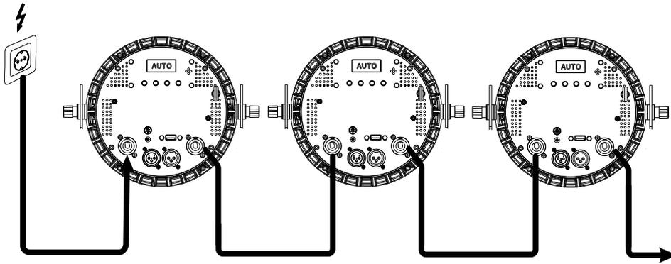
The device uses an auto-range power supply that accepts input voltages between 100 und 240 volts.
