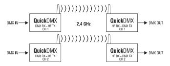
It is possible to operate 6 wireless DMX networks with 6 transmitters in parallel without mutual interference by adjusting them to different transmission channels. The wireless DMX networks operate independent of each other in 1:1 or 1:many transmission mode.
