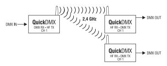
The DMX signal is fed to a transmitter which sends it via RF. Several receivers with the same transmission channel receive the RF signal and distribute it as a DMX signal.
