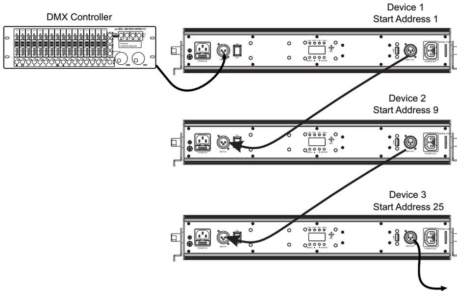
A DMX512 data link is required in order to control the device via DMX. The device provides 3-pin XLR connectors for DMX connection.
