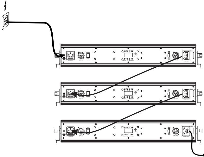
The device uses an auto-range power supply that accepts input voltages between 100 und 240 volts.
