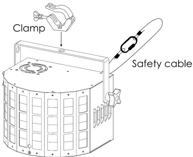
The Energetic can be placed on a flat stage floor or mounted to any kind of truss with a clamp.
