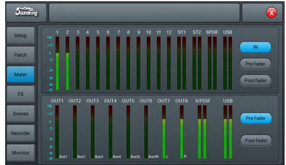
Signal level of input processing channel has three modes IN, Pre Fader and Post Fader with Pre Fader as the default. To select signal level mode to be displayed through single pressing the button. The signal level of output has two modes Pre Fader and Post Fader with Pre Fader as the default. To select signal level mode to be displayed through single pressing the button. On the right side of signal level of outputs you can see the bus names which are assigned to the port.
