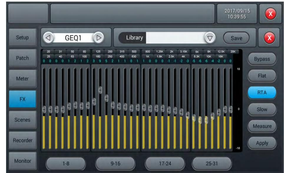
Please note that frequencies below 40Hz and above 16kHz are not automatically corrected, so you have to tune them manually.
