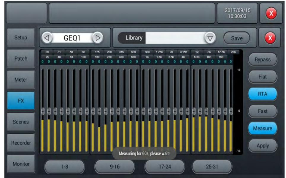
When the measurement is finished the Measure button will turn off. Now close the GEQ dialog and insert the GEQ in the LR bus either in the effects page or the input section of the LR bus. Then return to the GEQ, turn down the master fader and click apply, which will change your faders to equalize according to the last measurement.
