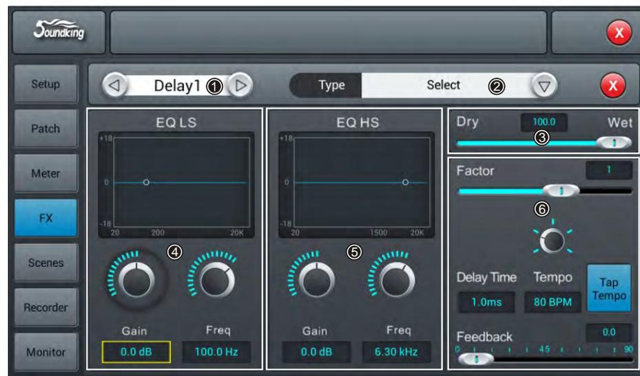
The Effects have 8 modules, which are 2 Modulation, 2 Delay, 2 Reverb and 2 15-band GEQ. All the modules can be inserted to input processing channel or bus processing channel, for one time only. Note, input processing channel can only be inserted with one effect module, while the bus can have two.
