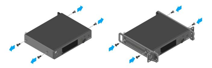
Secure the blanking plate to one of the mounting angles using two recessed head screws (M6x10).
