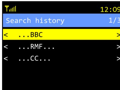
Turn the **TUNE/SELECT** control to choose the desired word or phrase and press the **TUNE/SELECT** control to confirm. The device will search for radio stations containing the chosen word or phrase.
