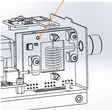
The evaporator can now be released by levering a small screwdriver through the two openings.
