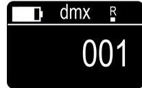
If a valid DMX signal is received, a small "R" appears above the quantity display.
