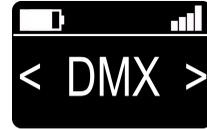
This can be changed using DMX address the minus button (9) and plus button (10). The address is automatically adopted after two seconds. This is indicated by flashing the address .
