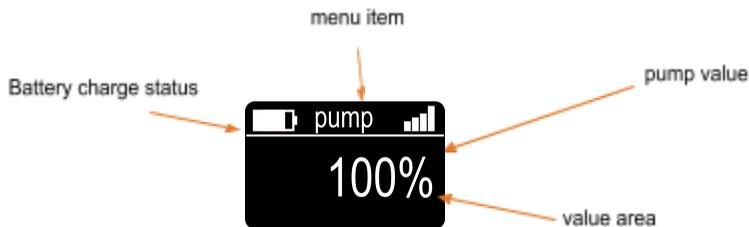
The operation of the Piccola takes place via the three buttons (minus / left, plus / right, enter) and the OLED display. In the upper part of the display, the charge status of the battery can be read on the left. The selected amount of fog is displayed in the upper right part. The selected menu item is displayed in the middle. The respective values are shown in the lower part of the display.
