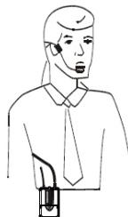
To use a "Lavalier" microphone connect the jack at the transmitter input.
