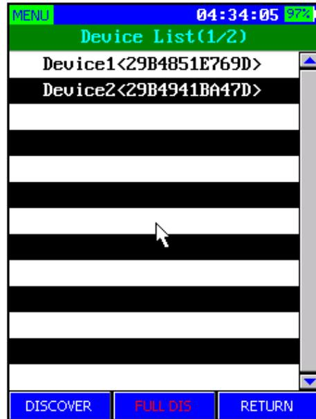
**FULL DIS** is full discovery. Using this option, any previously discovered list will be cleared, mute marks deleted, and it will discover all currently connected RDM fixtures. For the initial discovery process, you should use **FULL DIS**.
