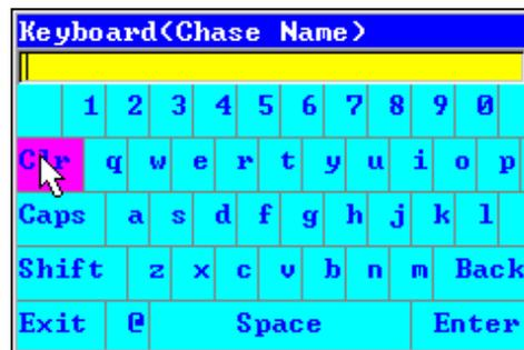
When input is complete, press **Enter**. To cancel an input, press **Exit**. If you need to input special characters, press **<@>** key (on the keyboard), to change the keys to symbols.
