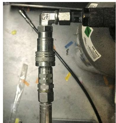
Open the CO2 bottle by turning the knob to the open side and make sure it is completely opened.
