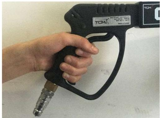
Turn the safety catch downward to lock the handle after use.
