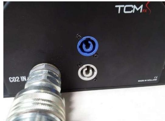
The Turbo Jet has a Powercon In and a Powercon Out connection. The blue Powercon connection is the power input. The grey connector is the loop through connector. By connecting a loop through to the output of the first Power Jet and the Input of the second Turbo Jet you can power multiple Power Jets to a single power socket.
