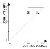
Here you can set up the transmission characteristic of your Dimmer pack. You can determine how control voltage (fader movement on the controller) is transmitted to the units connected in series. Depending on the mode, you can adjust a curve for all channels or for each channel individually.
