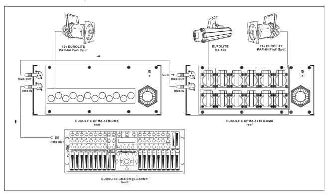
Connection example of the EUROLITE DPMX-1216 DMX and EUROLITE DPMX-1216 S DMX with the Controller EUROLITE DMX Stage Control, the theatre spots EUROLITE PAR-64 (dim mode) and the fog machine EUROLITE NX-150 (switch mode).
