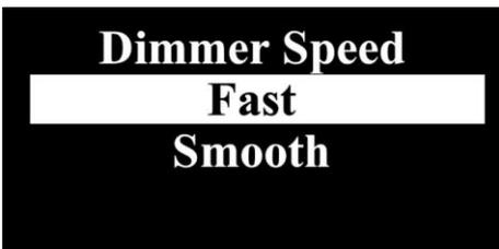
01) Press the **UP/DOWN** buttons to set the desired dimming speed. Choose one of the 2 options:
