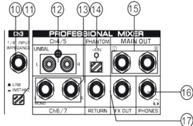
12.[TAPE/CD IN] TAPE / CD signal input jack.
