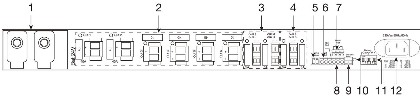
1.- Terminals for connection of the 24 V battery, type VRLA-AGM. The minimum charge that the battery can sustain for correct operation is 22 V provided that the connected equipment does not require more voltage.
