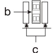
5.- **TEMP SENSOR:** signal input for a temperature sensor, euroblock terminals. This sensor must be placed between the batteries, in direct contact with both.
