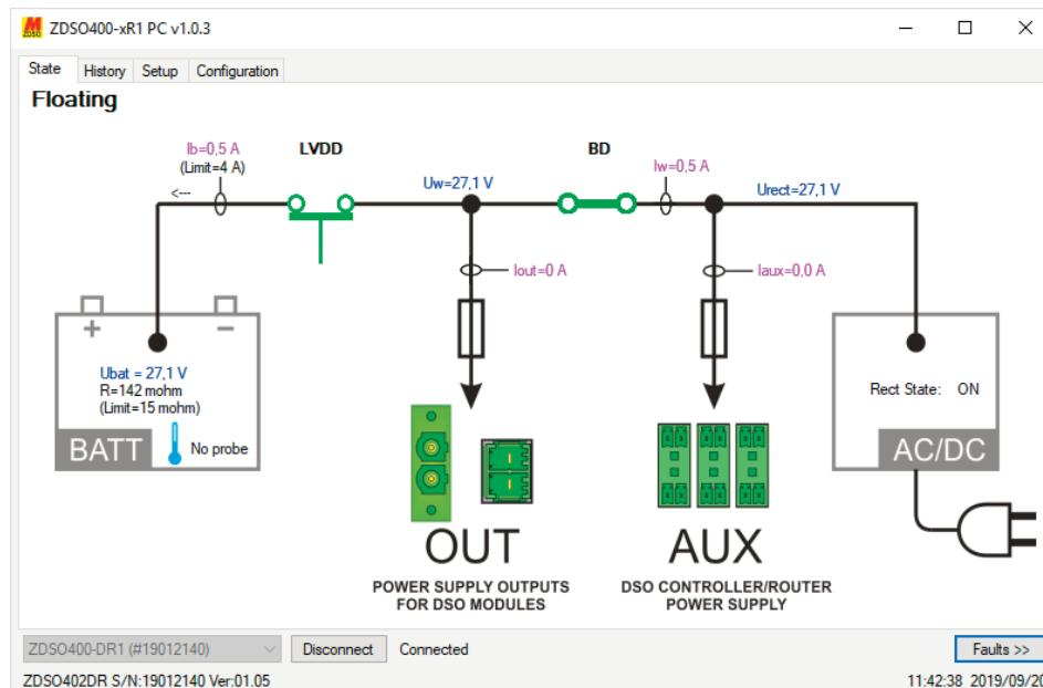
**LVDD** (Low Battery Disconnecting Device): protects against a total discharge of the battery.
