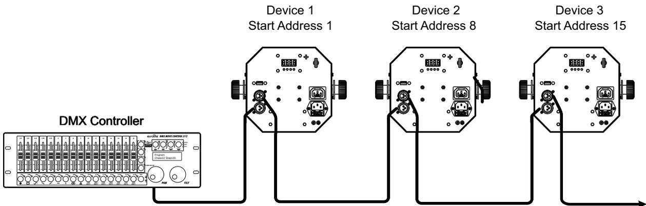
A DMX512 data link is required in order to control the device via DMX. The device provides 3-pin XLR connectors for DMX connection.
