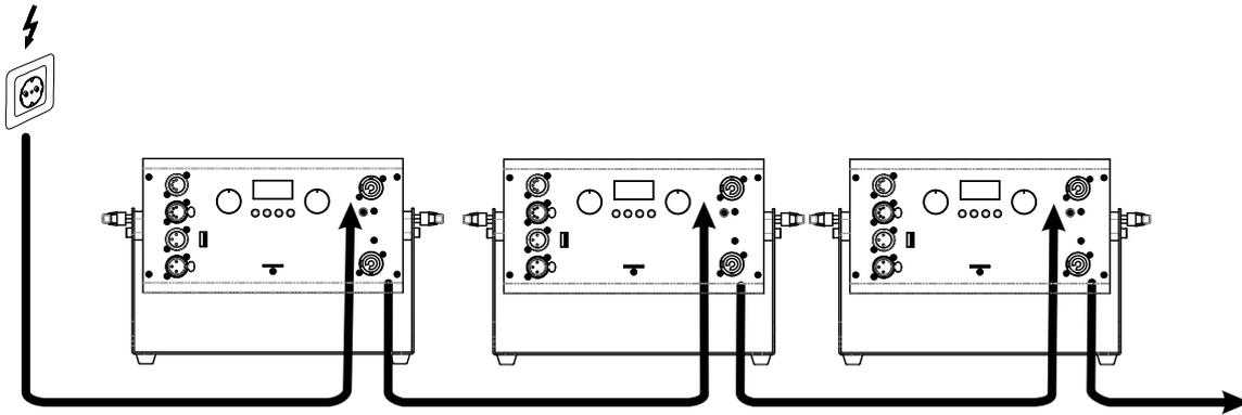
The device uses an auto-range power supply that accepts input voltages between 100 und 240 volts.
