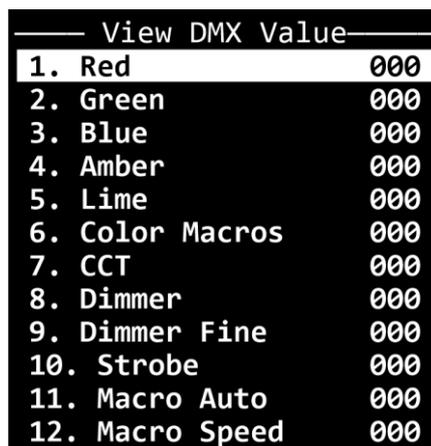
Depending on the selected DMX channel mode in the DMX Channel Mode submenu, you can see the following values:
