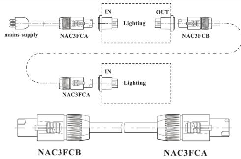
The power cable must is a three-conductor 2.5mm2 cable.
