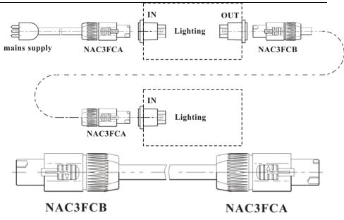
The power cable must is a three-conductor 2.5mm2 cable.
