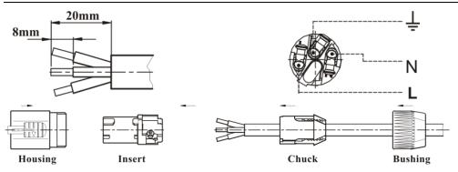
Put bushing and chuck onto the cable.
