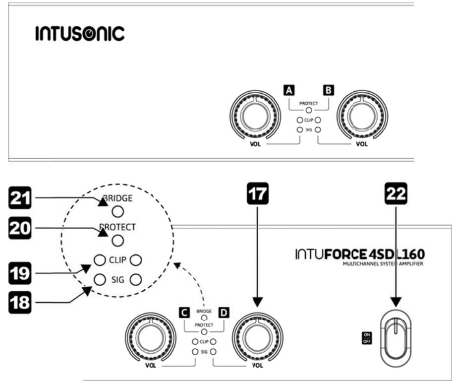
**17 Front Panel Channel Volume Control.** Set your desired output volume here for each of the 4 channels. Note that the maximum volume is set by the rear-panel maximum volume controls (8) and
