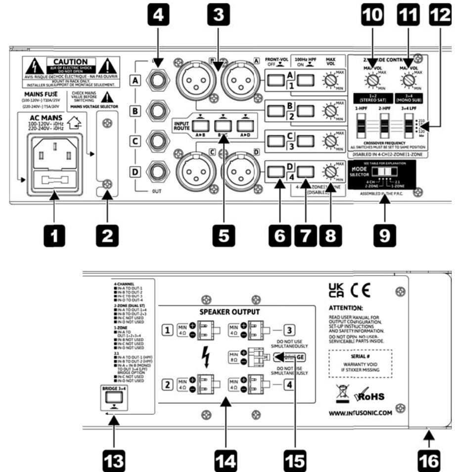
**1 AC inlet and fuse holder.** Use the supplied AC cord to connect the unit to AC mains. Make sure voltage and frequency stated and set on the unit comply with your local AC supply. The fuse can be accessed by the small drawer at the AC inlet. To change the fuse, unplug the AC cord first, pull out the fuse drawer and replace the fuse ONLY with a fuse of SAME voltage and rating. If the fuse blows again after replacement, hand over the unit to qualified service personnel.
