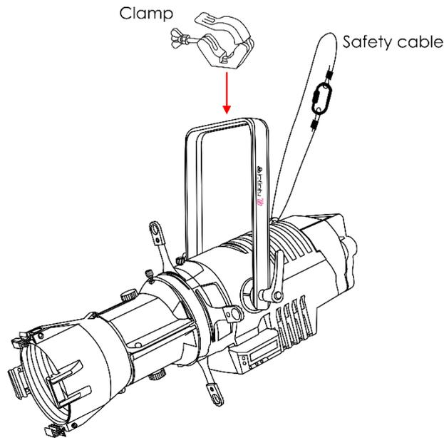
The Profile Engine TS-300 can be placed on a flat stage floor or mounted to any kind of truss with a clamp.
