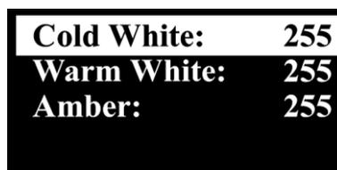
04) Press the **SETUP** button to confirm your selection and open the respective submenu where you can adjust the values.
