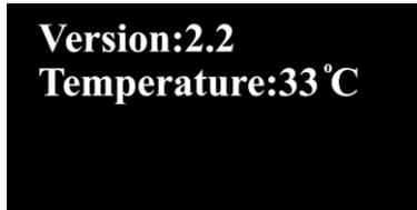
Immediately afterwards, the display will show the start screen (if the device is locked) or the main menu (if the device is unlocked). The start screen provides information about the operation modes of the device, the software version, the DMX channel mode and the temperature of the LEDs.
