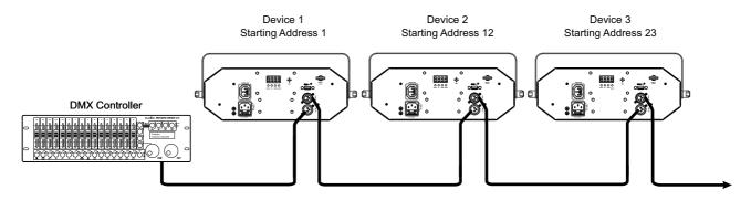
A DMX512 data link is required in order to control the device via DMX. The device provides 3-pin XLR connectors for DMX connection.
