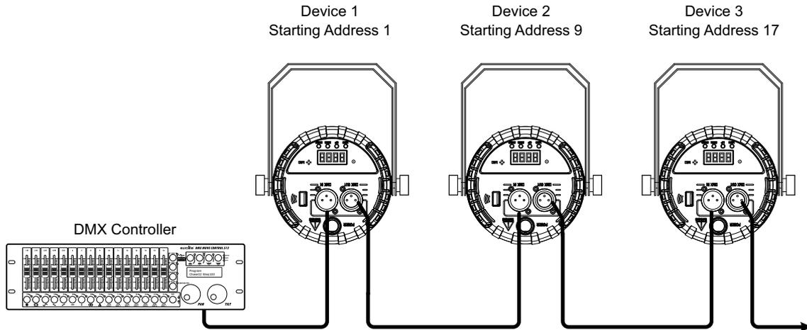
A DMX512 data link is required in order to control the device via DMX. The device provides 3-pin XLR connectors for DMX connection.
