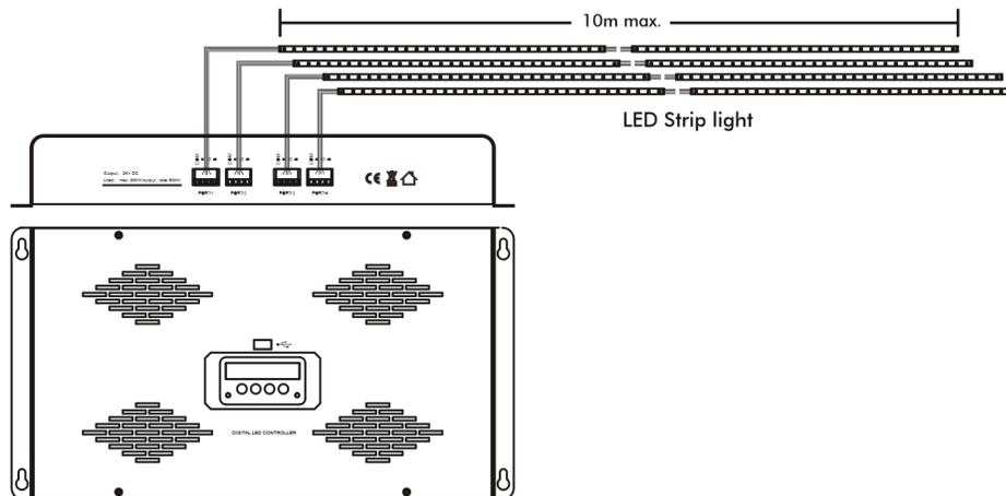
Connect the wires of LED strip to terminator of Ribbon Driver correctly base on color code of wire.
