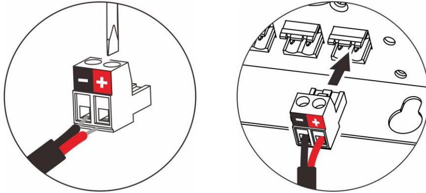
DarkFX Spot 510 IP is wired to output terminal of DarkFX Drive 4. Each output terminal can connect one DarkFX Spot 510 IP fixture.
