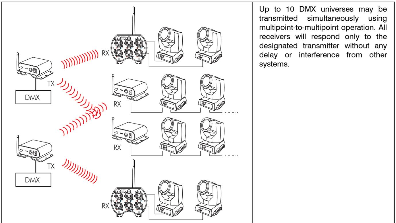
Up to 10 DMX universes may be transmitted simultaneously using multipoint-to-multipoint operation. All receivers will respond only to the designated transmitter without any delay or interference from other systems.
