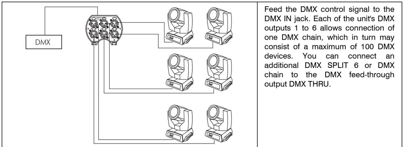
Feed the DMX control signal to the DMX IN jack. Each of the unit's DMX outputs 1 to 6 allows connection of one DMX chain, which in turn may consist of a maximum of 100 DMX devices. You can connect an additional DMX SPLIT 6 or DMX chain to the DMX feed-through output DMX THRU.
