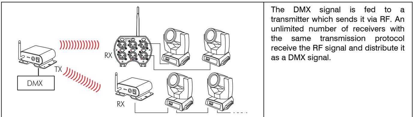
The DMX signal is fed to a transmitter which sends it via RF. An unlimited number of receivers with the same transmission protocol receive the RF signal and distribute it as a DMX signal.
