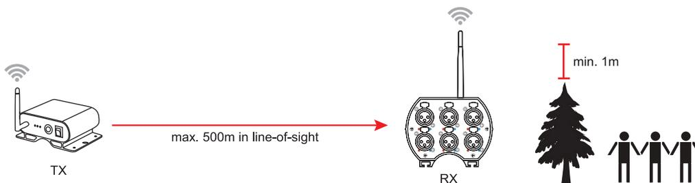
The maximum distance between the transmitter and receiver is dependent on the ambient conditions. To optimize range and performance maintain a line-of-sight between the transmitter and receiver and position the devices at least 1 m above the audience, trees and other obstacles.
