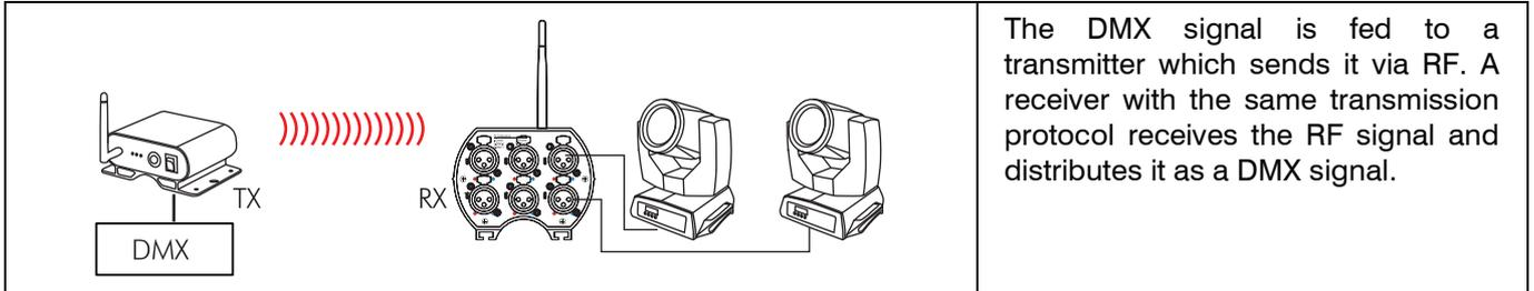
The DMX signal is fed to a transmitter which sends it via RF. A receiver with the same transmission protocol receives the RF signal and distributes it as a DMX signal.
