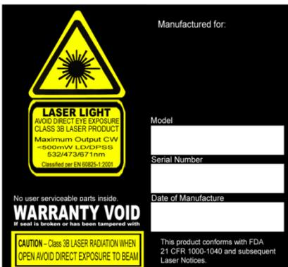
Combo label with the Product Model Number, Serial Number, Date of Manufacturing, Laser Light Warning Label, Warranty Void Label and Interlocked Housing Label
