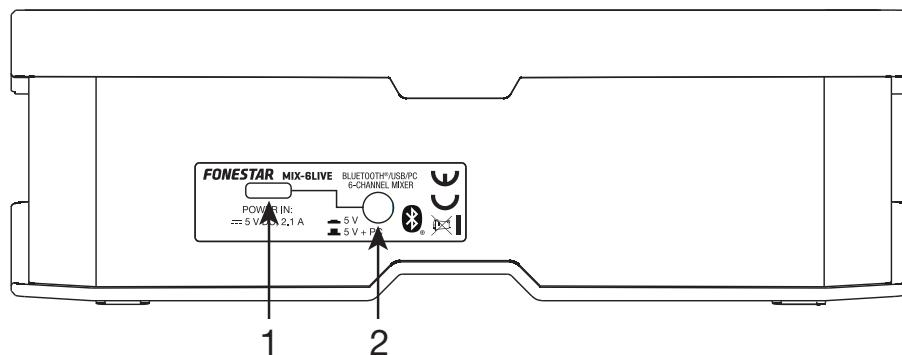
1.- Power and PC input. If a PC is connected with a USB cable this connection is for audio input and output or for control of the connected USB device. USB-C connector.
