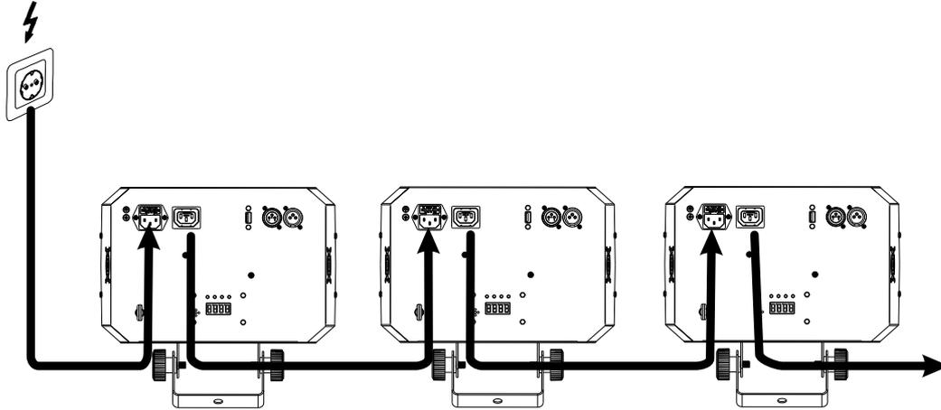
The device uses an auto-range power supply that accepts input voltages between 100 and 240 volts.
