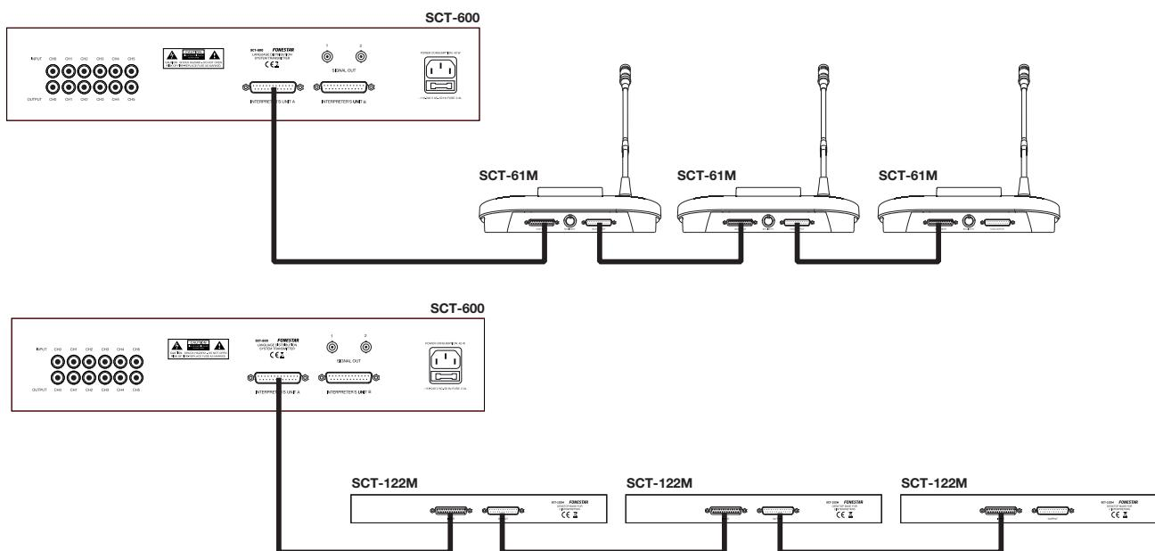
This equipment is supplied with a 10 meter long DB25 cable that can support up to 5 cascaded translation units. Increasing this length cannot ensure the proper functioning of 5 units.
